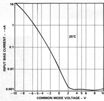
Figure 14. Input Bias Current vs. Common Mode Voltage
