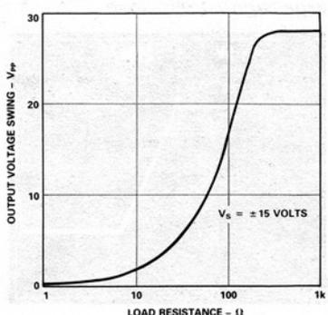
Figure 20. Output Voltage Swing vs. Load Resistance
