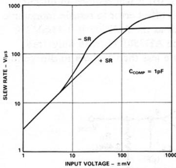
Figure 4. Slew Rate vs. Differential Input Voltage
