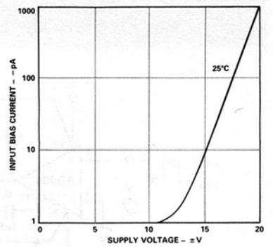
Figure 15. Input Bias Current vs. Supply Voltage
