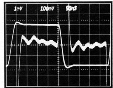
Figure 25c. Unity Gain Inverter Small Signal Response
