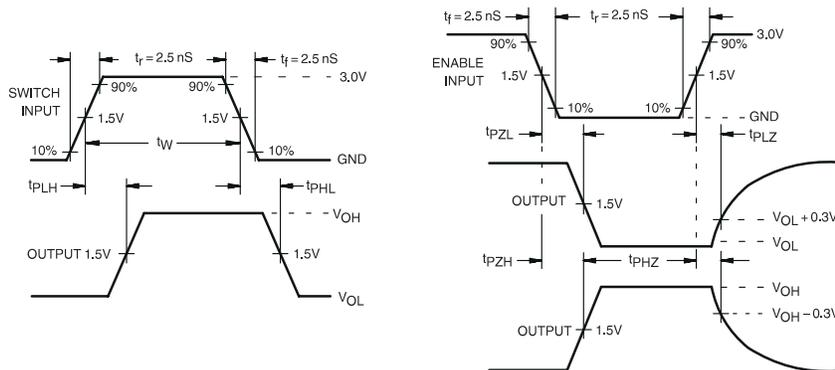
FIGURE 2. AC Waveforms
