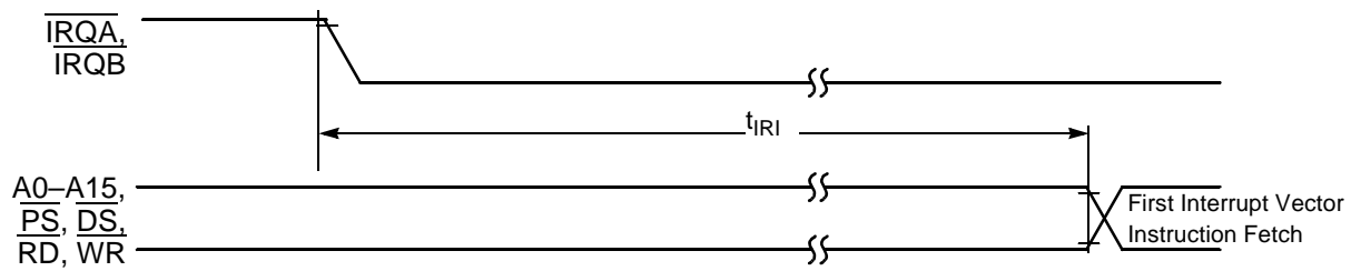
Figure 18. Interrupt from Wait State Timing
