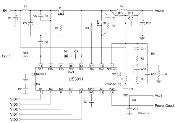
Typical application of US3011 in an on board DC-DC converter providing the Core supply for microprocessor.
