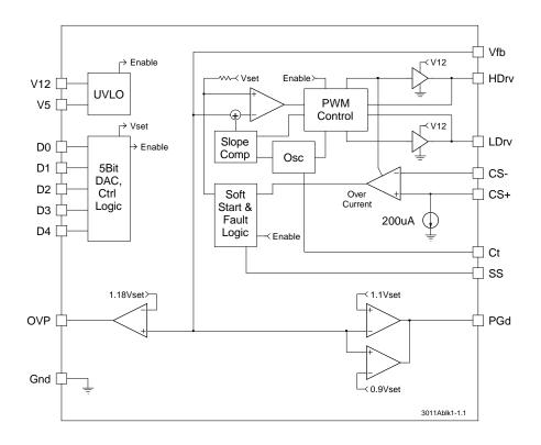
Figure 1 - Simplified block diagram of the US3011.
