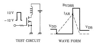
$\begin{array}{l} T_{ch} = 25^{\circ}\text{C (Initial)} \\ \text{Peak I}_{AR} = 5 \text{ A, R}_{G} = 25 \, \Omega \quad E_{AS} = \frac{1}{2} \cdot L \cdot I^{2} \cdot \left( \frac{B\text{VDSS}}{B\text{VDSS} - \text{VDD}} \right) \\ \text{V}_{DD} = 16 \text{ V, L} = 1.0 \text{ mH} \end{array}$
