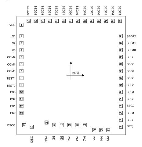
$<sup>\</sup>ensuremath{^{*}}$  The IC substrate should be connected to VSS in the PCB layout artwork.
