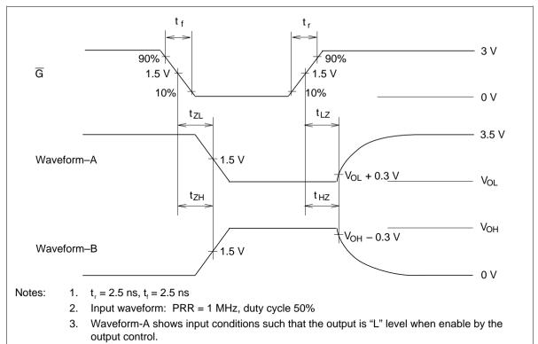
4. Waveform-B shows input conditions such that the output is "H" level when enable by the output control.
