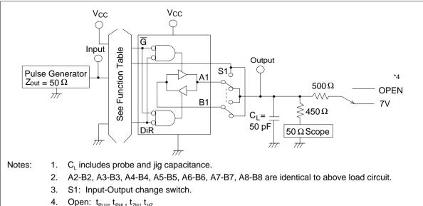
. Open:  $t_{PLH}$ ,  $t_{PHL}$ ,  $t_{ZH}$ ,  $t_{HZ}$ 7 V:  $t_{ZL}$ ,  $t_{LZ}$
