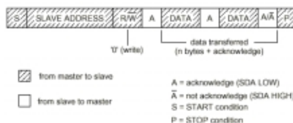
A master-transmitter addressing a slave receiver with a 7-bit address. The transfer direction is not changed.
