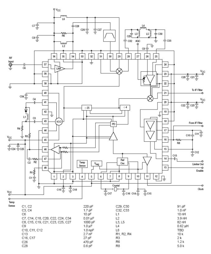
NOTES: 1. R8 must be set to match your 2nd IF filter impedance. 2. Layout of capacitors C10, C11, C12 is critical for stability of Limiter.
