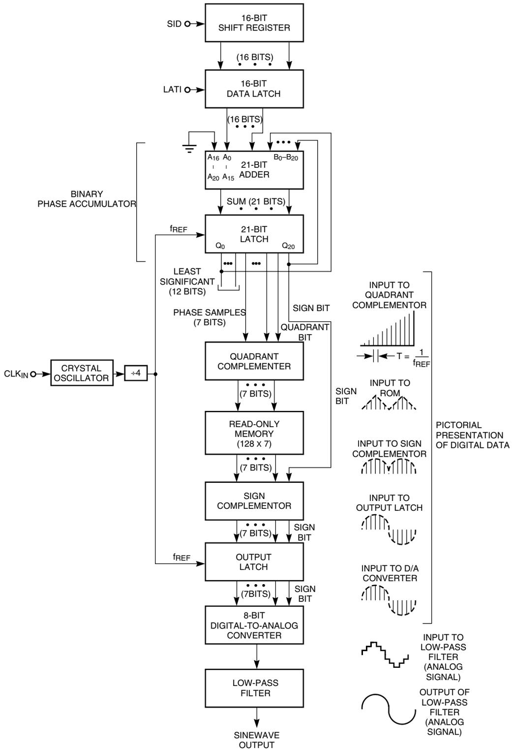
Figure 4. Detailed Block Diagram of the ML2036
