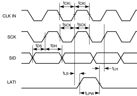
Figure 1. Serial Interface Timing.
