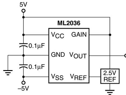
Figure 8. Sine Wave Generator with ± 2.5Vp-p.
