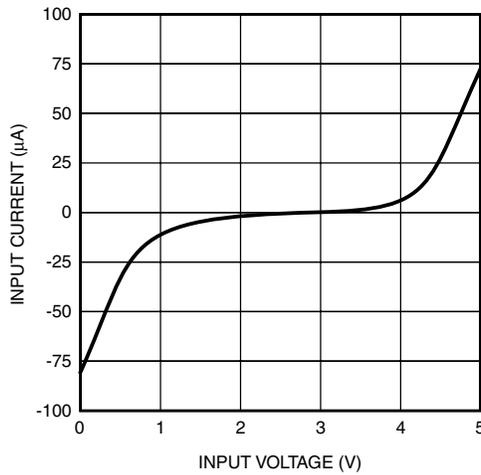
Figure 3. CLK IN Input Current vs. Input Voltage.
