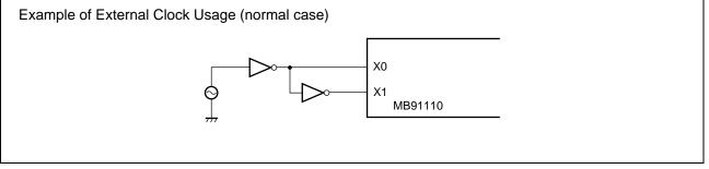
Note : Resistance must be added to the X1 pin if the STOP mode (oscillation stop mode) is used.
