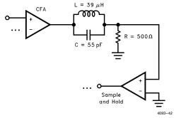
Figure 6. Colorburst Trap for NTSC Applications
