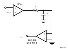
Figure 7. Caution: Lowpass Filter Does Not Work in NTSC Applications
