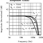
Frequency Response for Various  $R_F$  and  $R_G$
