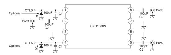
When using the CXG1008N, the following external components should be used:
