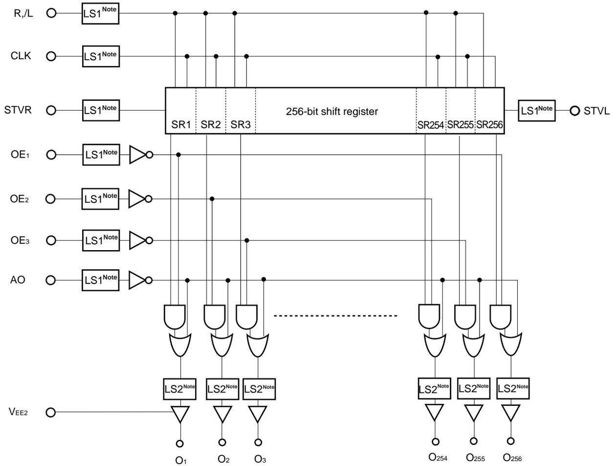
**Note** LS1: shifts CMOS level and internal level, LS2: shifts interval level and output level ( $V_{DD2}-V_{EE2}$ ).
