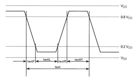
Figure 1 External Clock Input Waveform
