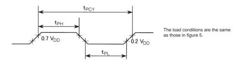
Figure 7 Port PE0 Pulse Output Timing
