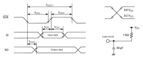
Figure 5 Serial I/O Timing
