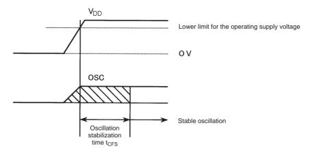
Figure 4 Oscillation Stabilization Time
