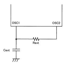
Figure 2 Two-Pin RC Oscillator Circuit
