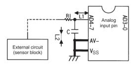
Figure 5 Analog Input Pin Wiring
