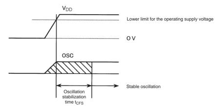
Figure 4 Oscillation Stabilization Time
