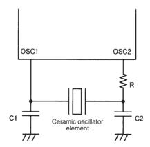
Figure 2 Ceramic Oscillator Circuit
