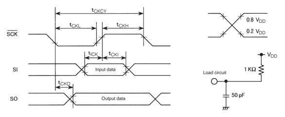
Figure 6 Serial I/O Timing
