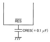
Figure 5 Reset Circuit
