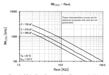
Figure 9 RC Oscillator Frequency Data (Representative Values)
