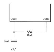
Figure 2 Two-Pin RC Oscillator Circuit
