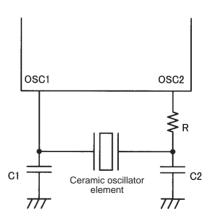
Figure 3 Ceramic Oscillator Circuit
