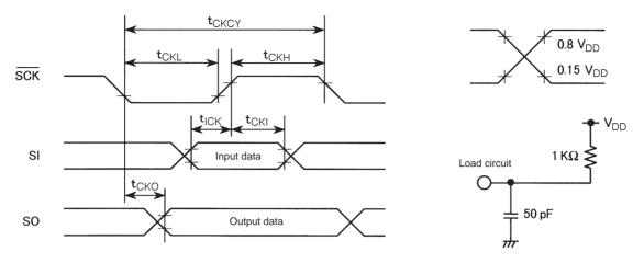
Figure 6 Serial I/O Timing
