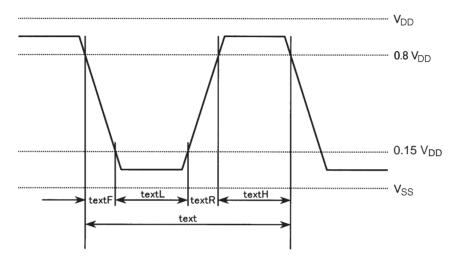
Figure 1 External Clock Input Waveform
