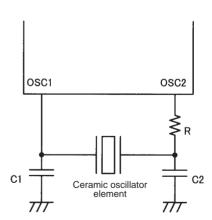
Figure 3 Ceramic Oscillator Circuit
