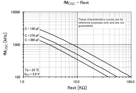
Figure 9 RC Oscillator Frequency Data (Representative Values)
