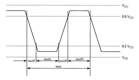
Figure 1 External Clock Input Waveform
