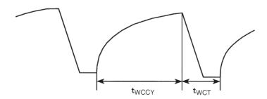
The charge time due to the time constant of the circuit consisting of the external components Cw, Rw, and Rl. The discharge time due to software processing. t<sub>WCCY</sub>:
