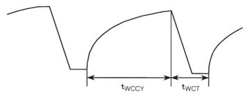
The charge time due to the time constant of the circuit consisting of the external components Cw, Rw, and Rl. The discharge time due to software processing. t<sub>WCCY</sub>:
