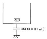
Figure 5 Reset Circuit
