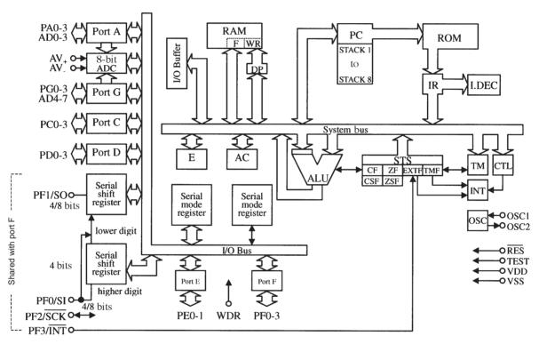
RAM: Data memory ROM: Program memory F: Flag PC: Program counter WR: INT: Working register Interrupt control AC: Accumulator IR: Instruction register ALU: Arithmetic and logic unit I.DEC: Instruction decoder
