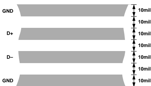
Figure 14. Arrangement of Signal Tracks
