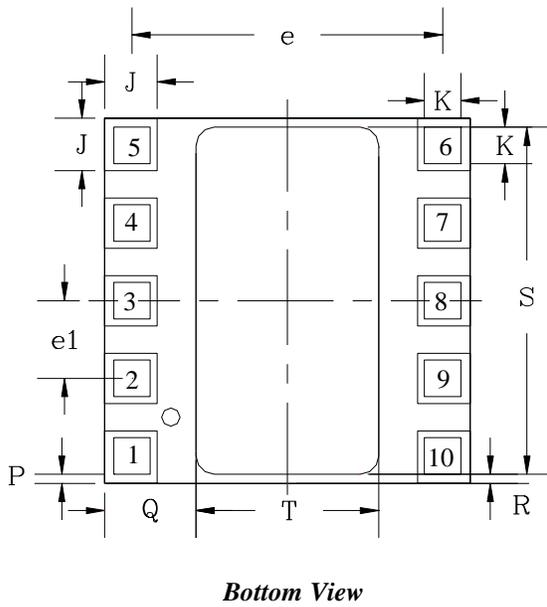
**Package Type: 10 Pin Plastic Module Package (cont'd)**
