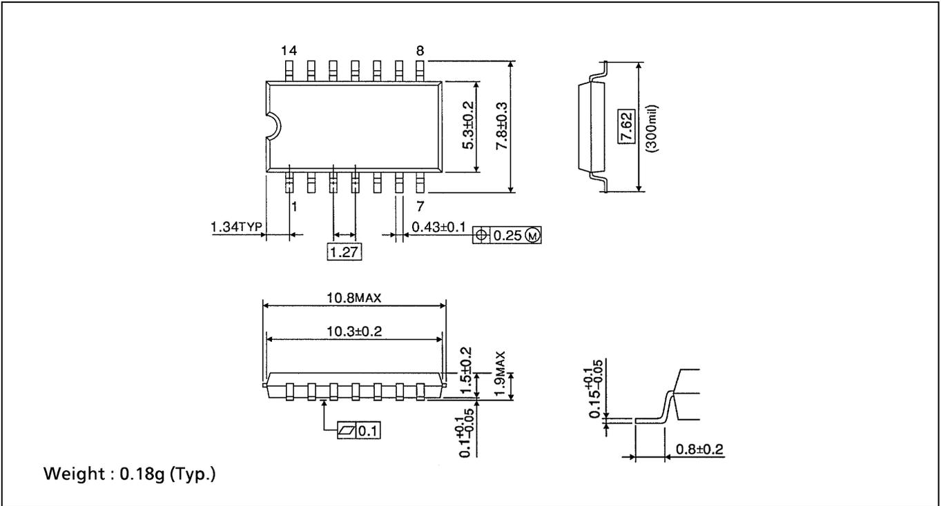
SOP 14PIN (150mil BODY) PACKAGE DIMENSIONS (SOP14-P-150-1.27)
