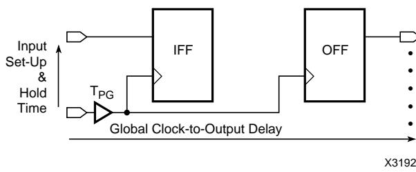
Timing is measured at pin threshold, with 50 pF external capacitive loads (incl. test fixture). When testing fast outputs, only one output switches. When testing slew-rate limited outputs, half the number of outputs on one side of the device are switching. These parameter values are tested and guaranteed for worst-case conditions of supply voltage and temperature, and also with the most unfavorable clock polarity choice.
