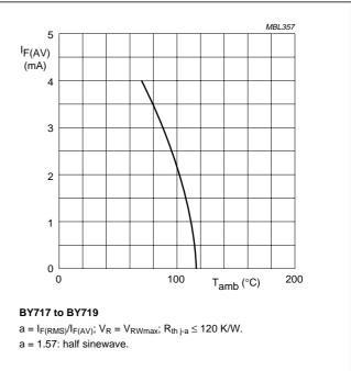
Fig.3 Maximum permissible average forward current as a function of ambient temperature.
