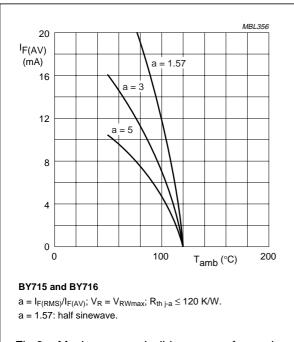
Fig.2 Maximum permissible average forward current as a function of ambient temperature.
