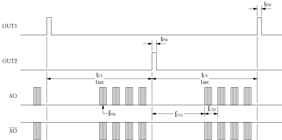
**Motor Output (Continuous Movement): CF5746BCA**
