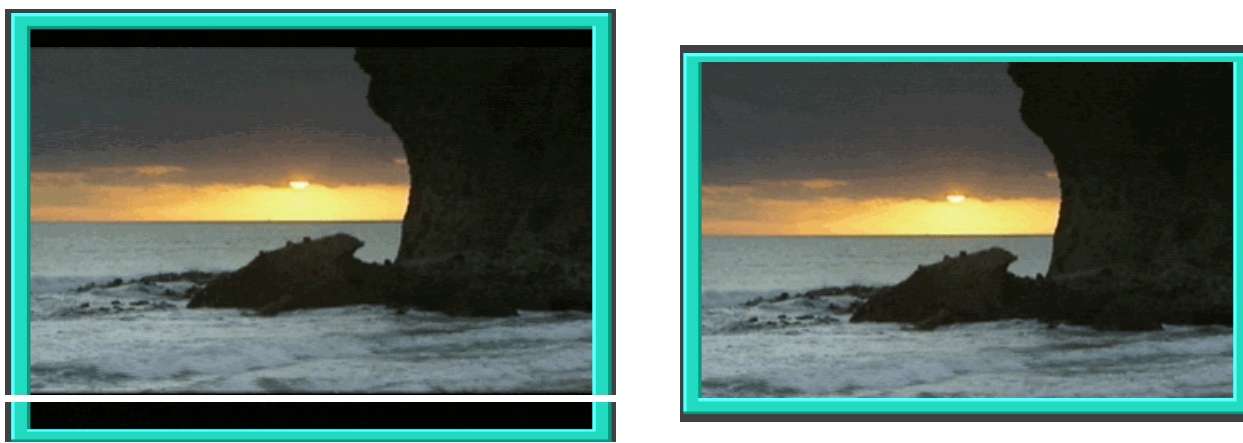
Figure 4-13 16:9 inset picture without and with reduction of vertical picture size
