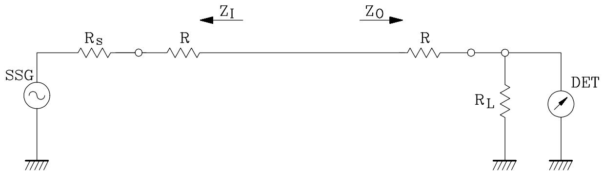
$R_S, R_L : 50\Omega$  (Internal Impedance of Source and Load)
