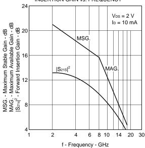
MAXIMUM AVAILABLE GAIN, FORWARD INSERTION GAIN vs. FREQUENCY **Gain Calculations**
