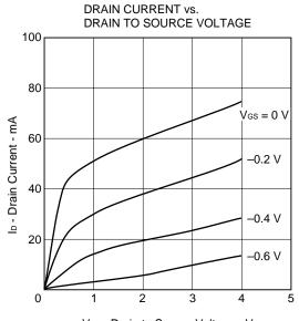
$V_{\mbox{\scriptsize DS}}$  - Drain to Source Voltage - V
