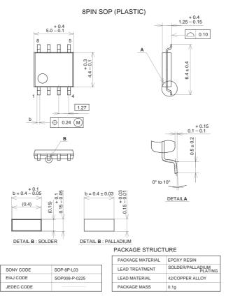
NOTE : PALLADIUM PLATING This product uses S-PdPPF (Sony Spec.-Palladium Pre-Plated Lead Frame).
