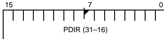
Figure 11-4 PIO Direction 1 Register (PDIR1, offset 78h)
