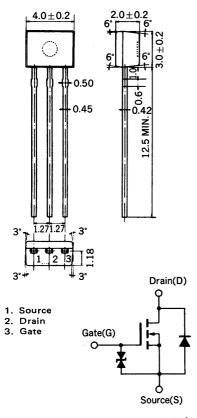
(Diode in the figure is the parasitic diode.)
