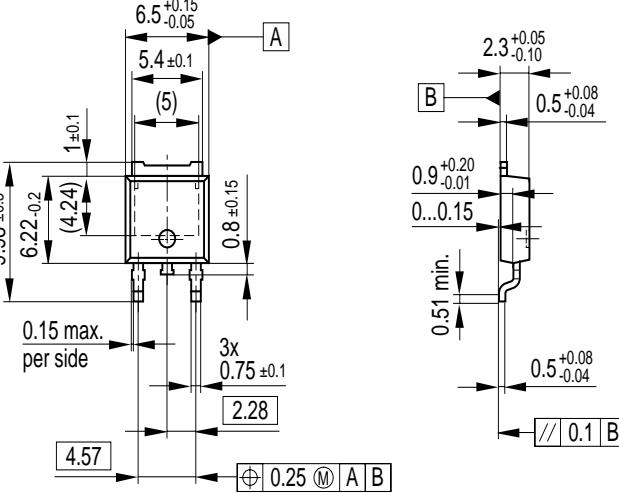
The drawing shows the physical dimensions of the package. Key dimensions include:
