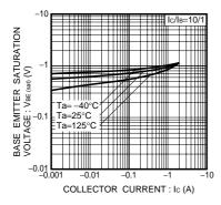
Fig.7 Base-Emitter Saturation Voltage vs. Collecter Current
