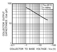
Fig.10 Collector Output Capacitance
