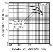
Fig.3 DC Current Gain vs. Collector Current (I)
